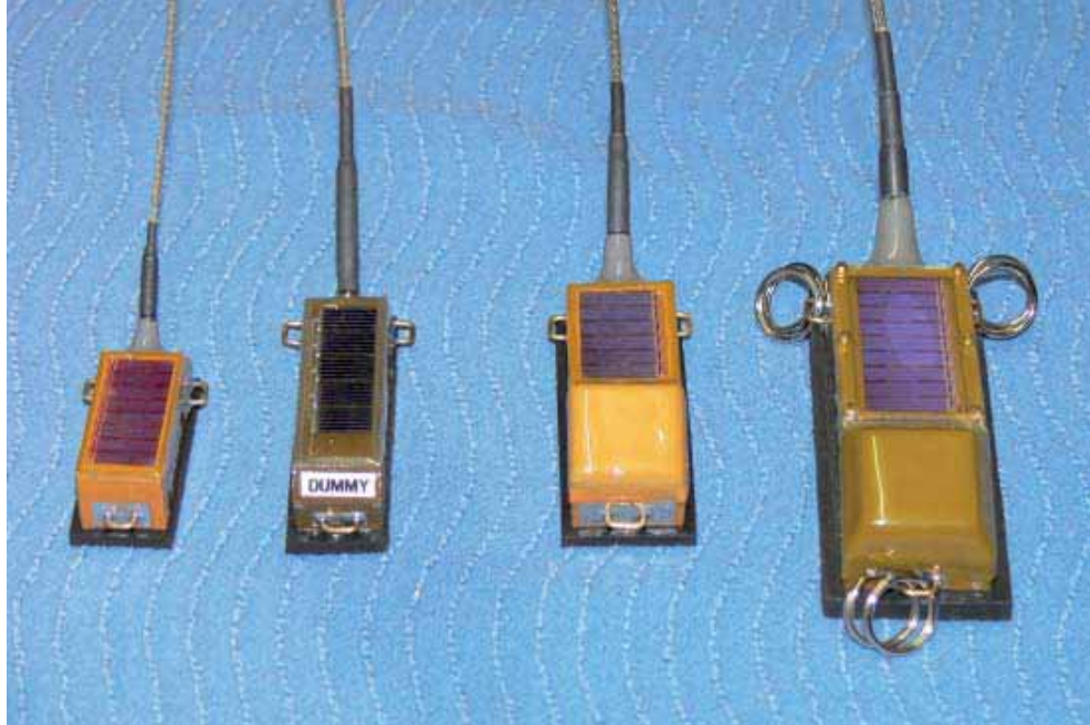
FIGURE 7.2 Platform terminal transmitters (PTT; three on the left); Global Positioning System (GPS) transmitter (one on the right)
