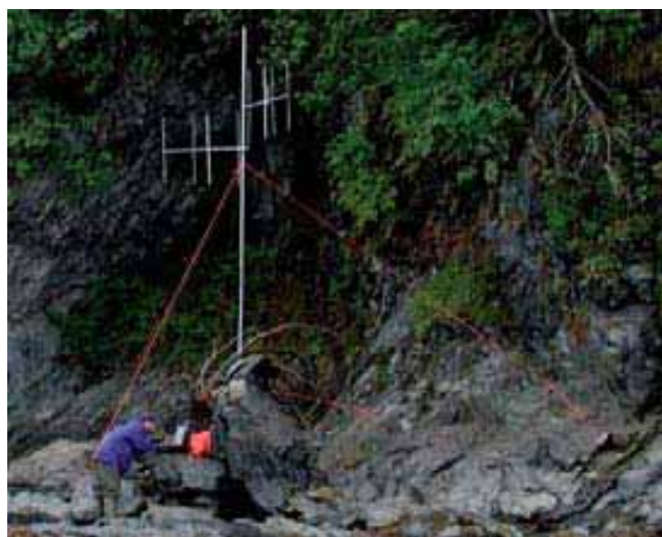
FIGURE 7.9 Yagi antennae mounted on a tower at a remote tracking station attached to a data logger
